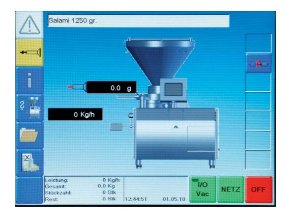
The ultimative stuffer control system with all variety of functions consists of an industrial personal computer and a touch screen panel in the front door of the filling machine.
